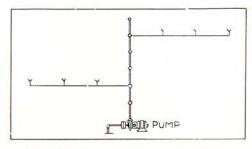
Sprinkler line moved to second position. If your crop and soil will take the water fast, a 40 x 40-foot sprinkler setting without staggering can be used and moved often. If the opposite is true of your crop and soil, a 60 x 60-foot sprinkler setting can be used if staggered at each move. Each system has its merits. Let us recommend. The sprinkler coverage circles inter-lock so that uniform irrigation is given over the entire field.
