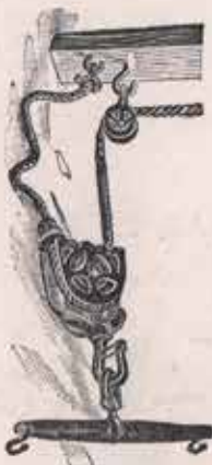
Fig. 135—Porter Snatch Pulley Block Weight—5½ pounds. Frame—Certified malleable iron. Sheave—Gray iron. Shortens distance team must travel in elevating load. By slipping washer on the rope and tying a knot just behind it the rope can be thrown off the pulley, and the empty fork returned without waiting for team to get back to barn.
