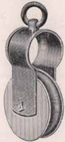
No. 144 represents our Steel Frame Knot Passing Pulley with 6-inch maple sheave and 1-inch pipe bushing. No. 143—Same as above but not knot passing. Weight, 40 lbs. per doz.
