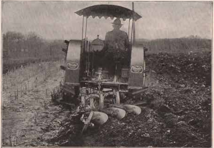
Heider 12-20 and Rock Island No. 19 Power-Lift Plow Turning an Acre an Hour
