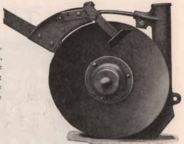
Disc Shoe, Showing Concave Side of Disc
