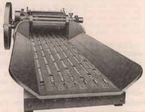
View Showing Grip Hook Table and Channel Iron Apron on Smalley Alfalfa Cutter
