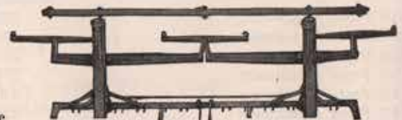
Three-Horse Chain Equalizer Hitch, Two Poles
