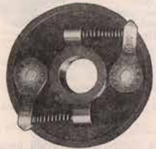
Wheel Clutch Placed on Outside of Axle—Easy of Access
