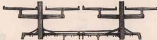
Four-Horse Chain Equalizer Hitch, Two Poles
